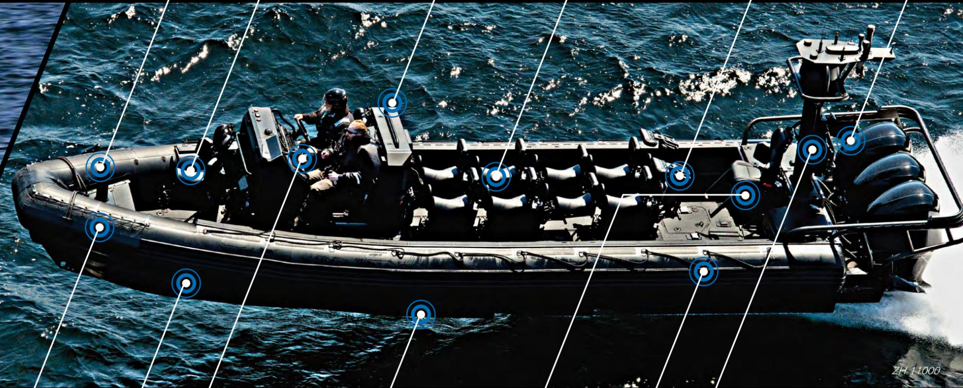
Twin stern drive propulsion system    Removable weapon mounts    Deck track for easy re-configuration    Futura Commando Boat deployment platform    Double inboard diesel Engine    Double console: Navigation & Command    Weapon mount    Bow & AFT boarding pole    Shock Mitigated console & climate control radio box    12 x Milpro Air Shock Mitigating seats    Recessed deck tracks for easy re-configuration    Triple Outboard gasoline engine
